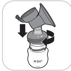
3. Screw the pump body onto the bottle.
