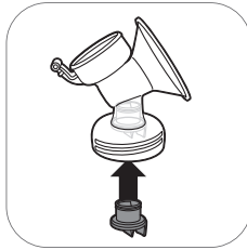
2. Push the white valve in the pump body as far as possible.
