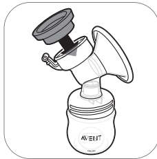
5. Place the silicone diaphragm in the pump body.
