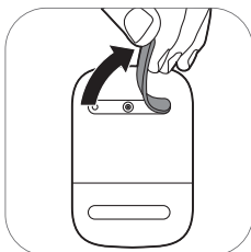
1. Remove the rubber feet from the bottom of the motor unit.
