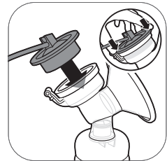
6. Attach the silicone tube and cap onto the silicone diaphragm. Push down the cap until it is securely in place.
